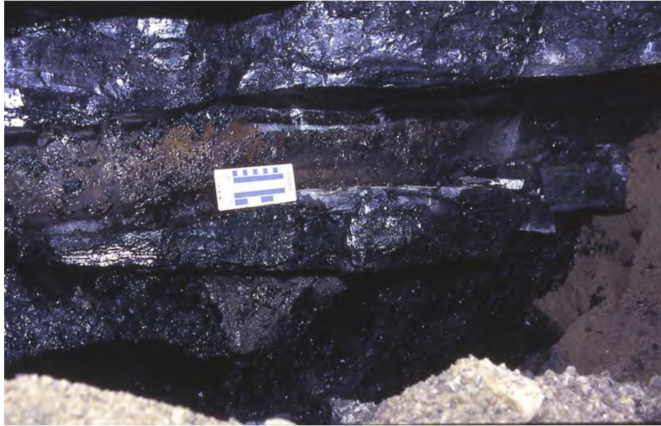
Figure B.8 Massive segregated ice in bedrock (coal layers), Ellesmere Island (See Clause B.2.4.)
