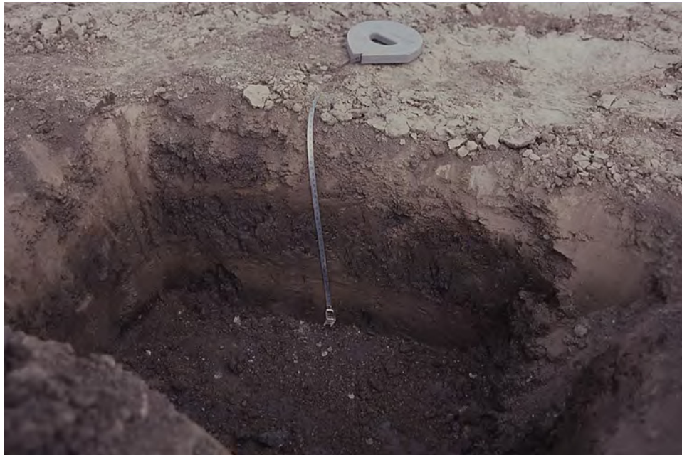
Figure B.5 The active layer exposed in a soil pit on Ellesmere Island (See Clause B.2.3.)
